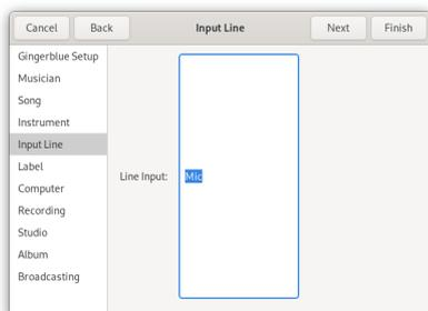
Type the name of the audio line input. The default audio line input is “Mic” ( `gst_pipeline_new("record_pipe")` in GStreamer). Click “Next” to continue ((or “Back” to start all over again) or “Finish” to skip the details).
