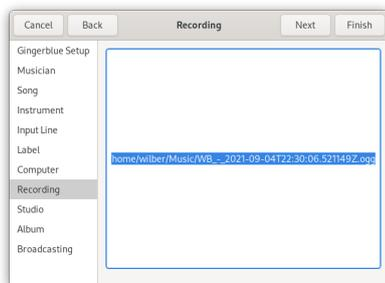
Notice the immediate, live recording file. The default immediate, live recording file name falls back to the result of `g_strconcat(g_get_user_special_dir(G_USER_DIRECTORY_MUSIC), "/", gtk_entry_get_text(GTK_ENTRY(musician_entry)), "_-", gtk_entry_get_text(GTK_ENTRY(song_entry)), "_[", g_date_time_format_iso8601 (datestamp), "]", ".ogg", NULL)` in `gingerblue/src/gingerblue-main.c`
